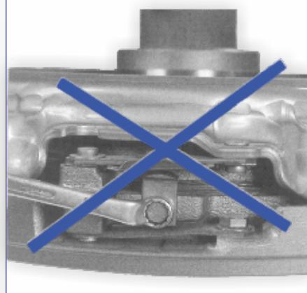
**FAULT:** Clutch doesn't separate (double pull clutch)
