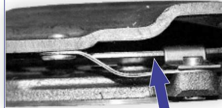
**FAULT:** Clutch does not separate.
