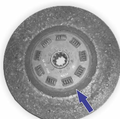
**FAULT:** Excessively worn out clutch disc facing by the flywheel.
